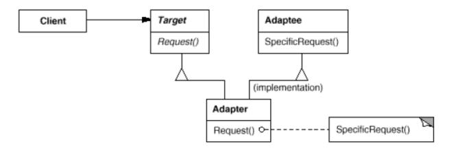
An object adapter relies on object composition. The structure of an object adapter is as shown below:
