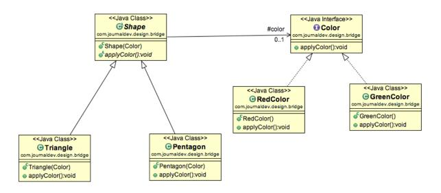
Notice the bridge between Shape and Color interfaces and use of composition in implementing the bridge pattern.
