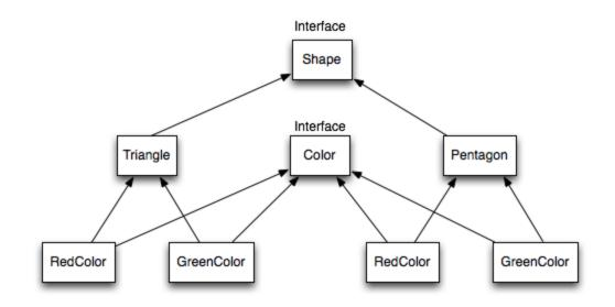
Now we will use bridge design pattern to decouple the interfaces from implementation and the UML diagram for the classes and interfaces after applying bridge pattern will look like below image.
